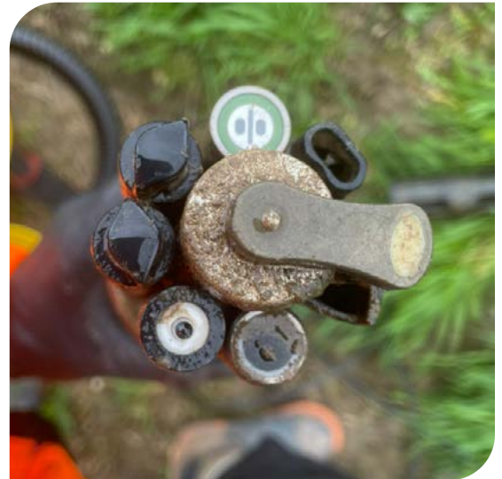
The EXO Central Wiper reduces fouling on the sensor faces, while the Ammonium ISE wiper guards protect the ISE membranes.
