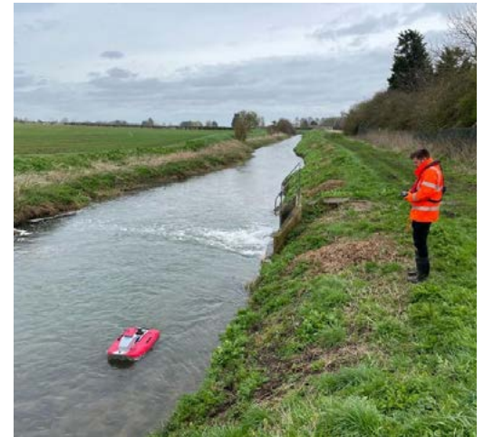
Figure 1. An example showing how the wastewater outfall location is evident from the distribution of spatial ammonium concentration data collected during a one-time survey performed with an rQPOD Remote Surface Water Vehicle equipped with an EXO Sonde.
